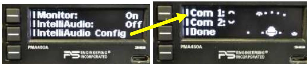
Figure 3-3 IntelliAudio – True Dimensional Sound, Spatial Location Display, showing C1 at 30°left and C2 at 90° right of center.
