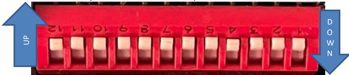
Switch going towards the number is "UP" Switch going away from the number is "DOWN"
