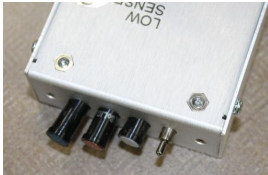
Figure 2-3 - MB10 with lamps extended for installation
